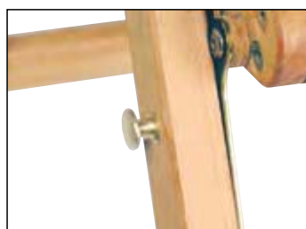
Close up of locking pin
