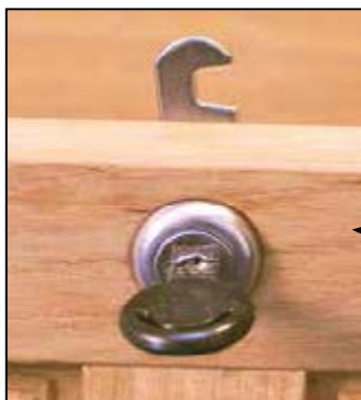
Close up of Cam lock
